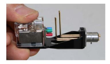
**4. Bend red & white leads upward.** Bend white and red leads upward about 1/4-inch (6mm) before the cartridge.
