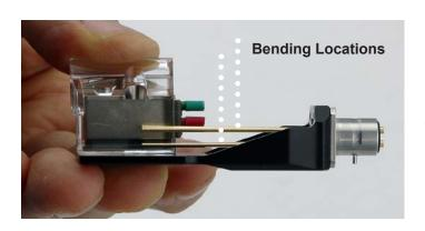
**2. Hold cartidge next to leads.** Temporarily position the cartridge next to the leads to estimate the required lead lengths.
