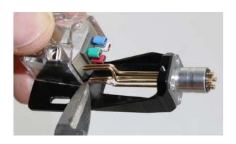
**6. Trim leads.** Trim the leads with wire cutters at the appropriate lengths for the cartridge connections.
