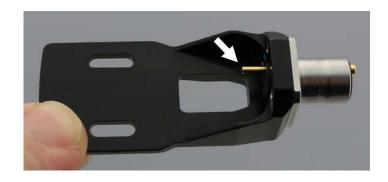
Once the leads are cut and inserted, attach the standard flexible wire leads to the remaining stubs.
