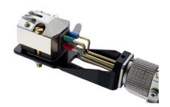
Insert leads through the head shell connector. The thinnest end of the lead must be pushed through the connector.
