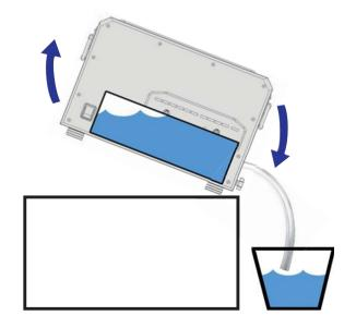
Once the reservoir is completely empty, unscrew the rear access cap. If the unit will be shipped or transported, paper towels can be placed inside the reservoir to absorb residual water (along with replacing the access cap).
