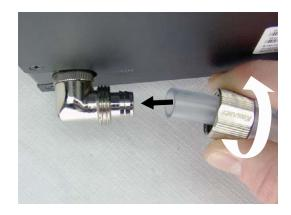
To drain, push the included PVC tubing onto the barbed fitting marked "Drain" and screw on the knurled compression ring. Position the opposite end of this tubing into a sink or large container to capture the older water.
