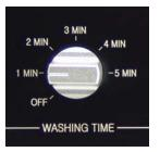
"WASHING TIME" adjusts the ultrasonic washing time from 1-5 minutes. Longer cleaning times are intended for especially difficult-to-clean records. It is suggested to start with a short time period and increase if needed. If only drying is desired, select "OFF".
