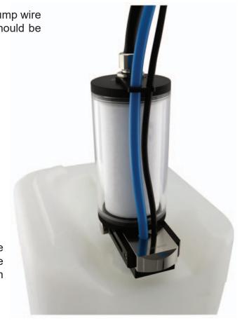
An extra replacement filter is provided, and more are available from Klaudio. Access the filter core by unscrewing either end cap from the housing. A strap wrench can be used if needed.
