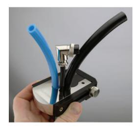
The filter will be located on the black supply tubing. It can be attached directly to the reservoir mounting bracket, or placed elsewhere on the tubing. The filter can operate in a vertical or horizontal orientation.
