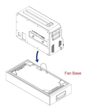
**Step 5:** Place the record cleaner onto the fan base. When properly aligned, it should fit firmly and level.
