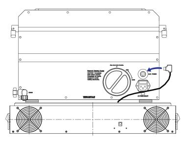
**Step 6:** Connect the fan power plug from the base to the record cleaner's "Aux Power" port. Optionally, the fans can be powered with a separate supply via the barrel plug near the fan grills (12VDC, 0.5A).
