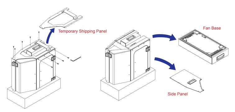
**Step 1:** Remove right half of foam packaging and peel back the vinyl bag to expose temporary shipping panel. Unscrew panel with the provided hex wrench.
