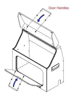
**Step 4:** Attach handles to top and front doors with the provided hardware and phillips screws.
