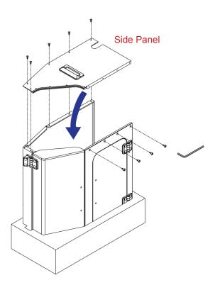
**Step 3:** Attach side panel to the silencing box with the original hex screws and wrench.
