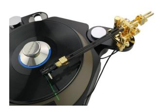
Klaudio models KD-ARM-AG10 (10.5-inch equivalent) and KD-ARM-AG12 (12-inch equivalent) tonearms add automatic lift and electronic descent features to the tangential lineup. The arms can be dropped or raised at the press of a button, and they automatically lift at the end of playback. These versions are gold plated with carbon fiber arms.
